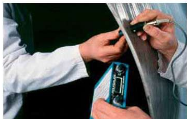
Ultrasonic Thickness Test
