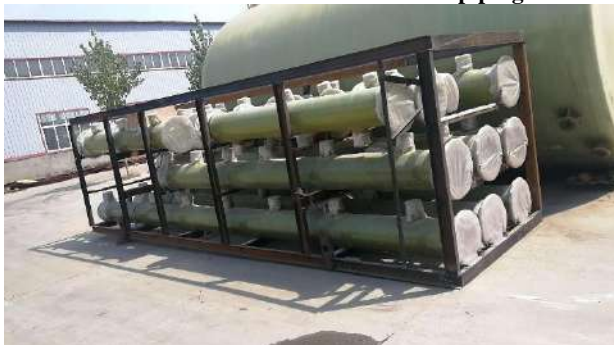
Full vacuum FRP piping for a hot acid WesTech project in Morocco:
