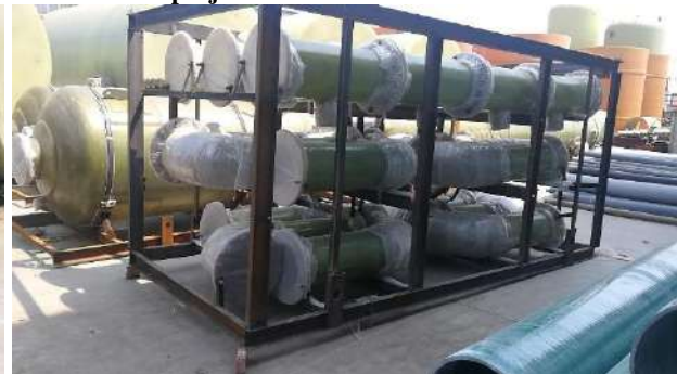
Full vacuum FRP piping for a hot acid WesTech project in Morocco:
