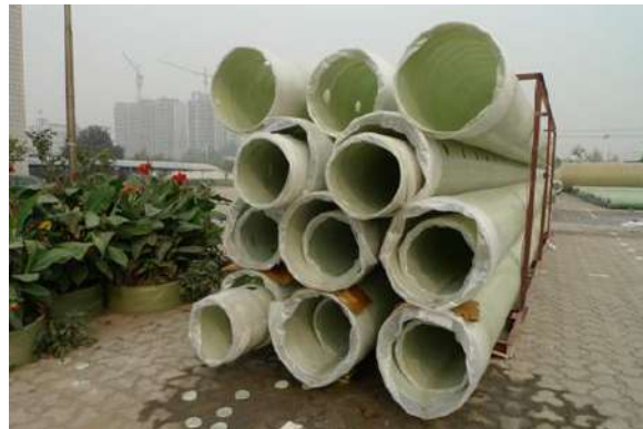
Full vacuum FRP piping for a hot acid WesTech project in Morocco:
