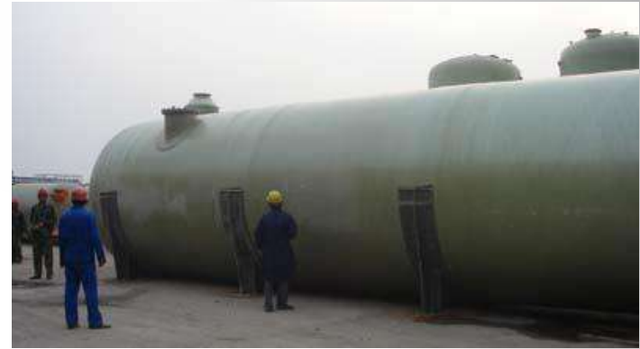
Polyethylene liner and completed PE lined FRP vessel
