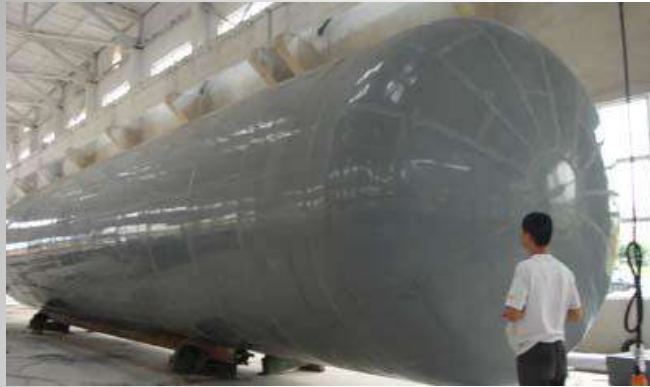
Polyethylene liner and completed PE lined FRP vessel
