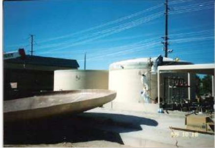
28' x 12" acid storage made in Texas, shipped to Arizona
