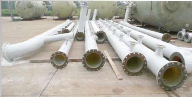
Prefabricated piping system for Phelps Dodge
